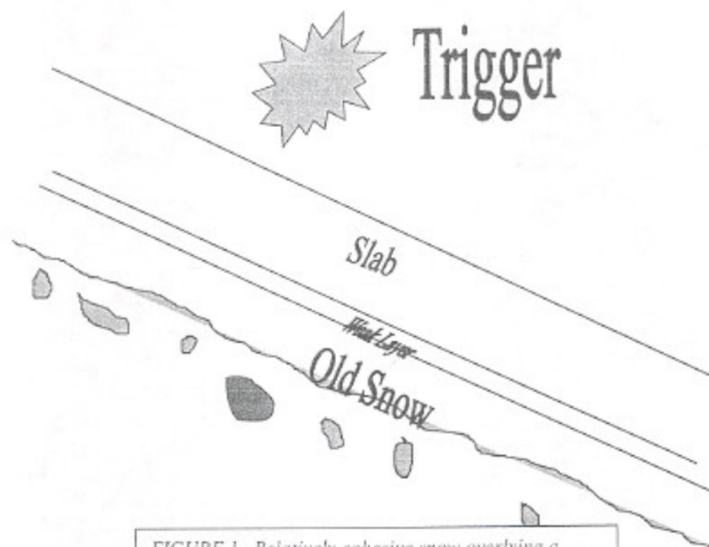
FIGURE 1. Relatively cohesive snow overlying a weaker, less cohesive layer constitutes a slab.
